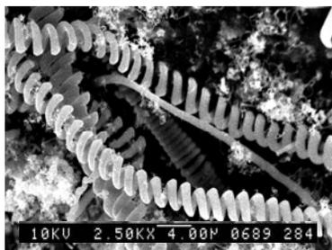
Fig. 4. Regular single-helix carbon nanocoils. Catalyst: Fe-Cr- Ni.
