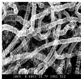
Fig. 8. Carbon microcoils with large coil diameter. Reaction temperature: 750° C, by WS<sub>2</sub> catalyst
